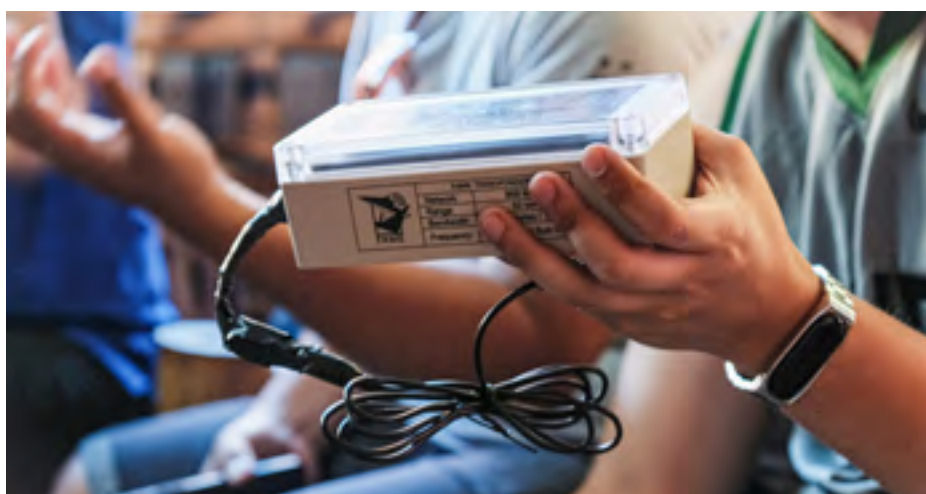
A Vessel Monitoring Measure (VMM) provided by Futuristic Aviation and Maritime Enterprises (FAME). Portable and affordable, it can help authorities track fishing activities, allowing for better management of Philippine fisheries.
